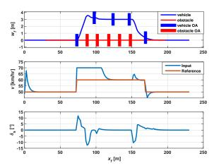
Fig. 4. Final vehicle control performance obtained by the designed MPC controller. The top subplot shows the vehicle and obstacle positions. The "vehicle OA" and "obstacle OA" bars show five relative positions of the vehicle and obstacle during the OA period. The middle subplot shows the actual and reference velocity v at different longitudinal positions. The bottom subplot shows the steering angle  $\psi$  over the longitudinal position.
